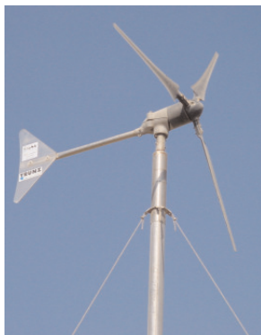
Windgenerator Max. 1'000 W/h
