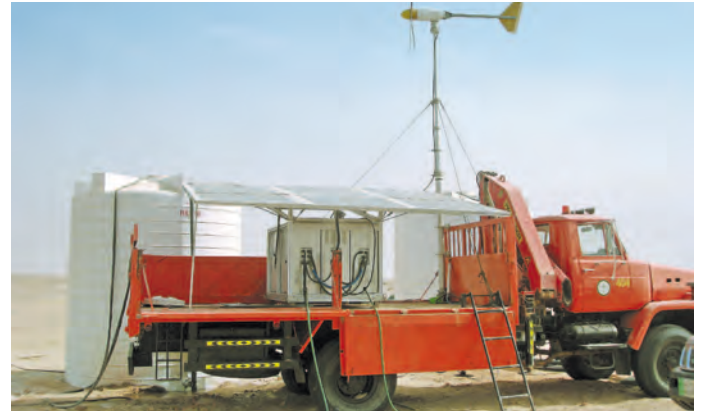
TSS 200: treatment of brackish water incl. wind generator in the desert of Abu Dhabi, 2010
