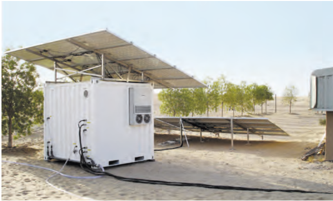
TBC 100: solar powered brackish water container located in the desert, Abu Dhabi 2009
